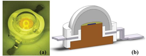
Fig. 3. (a) Picture of typical LED module and (b) its corresponding model.
