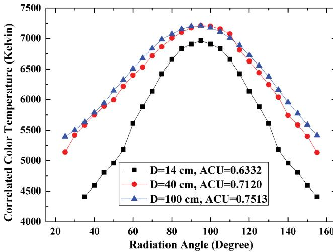
Fig. 4. CCT variation of typical leadframe LED module in the experiments.
