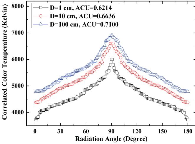
Fig. 5. CCT variation in the whole radiation angle in the simulations.
