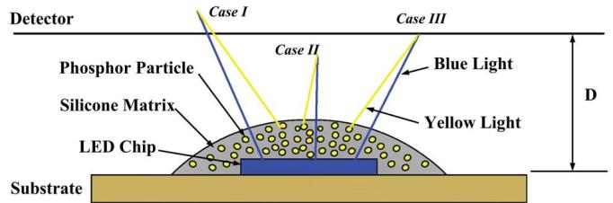
Fig. 1. Schematic of white light generated by color mixing.
