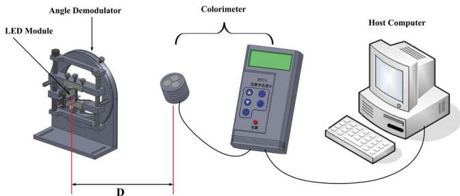
Fig. 2. Configuration of experimental apparatus.
