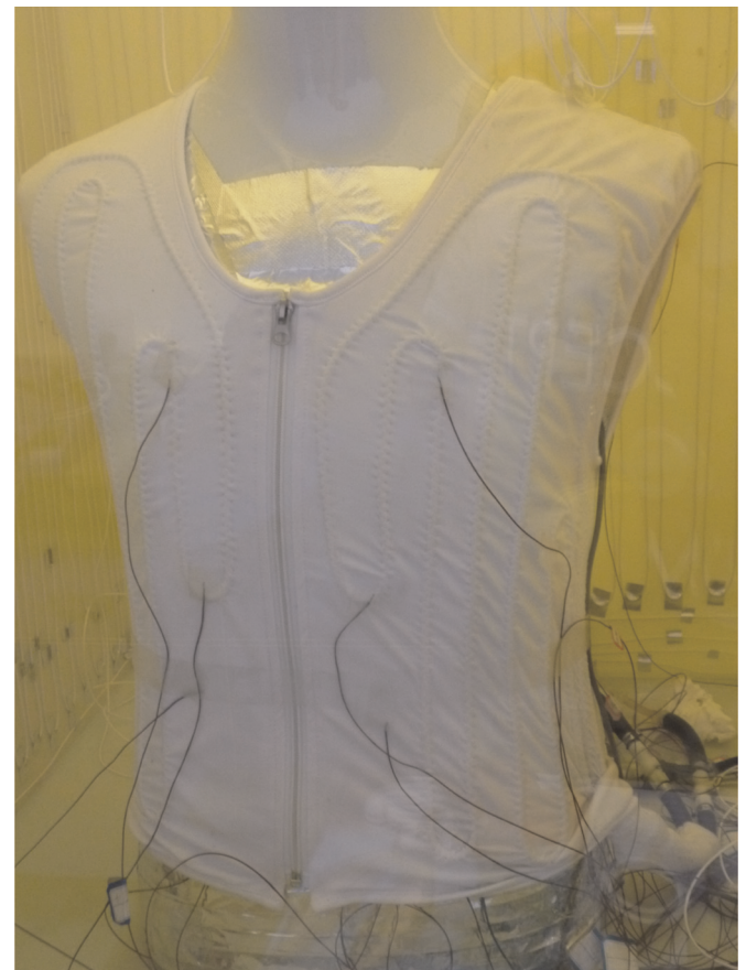
Fig. 3. The photo of the prototype of LCG on the manikin. Cooling tubings were sewed to the lightweight basic garment and a zipper was used to make the LCG easy to take on and off.
