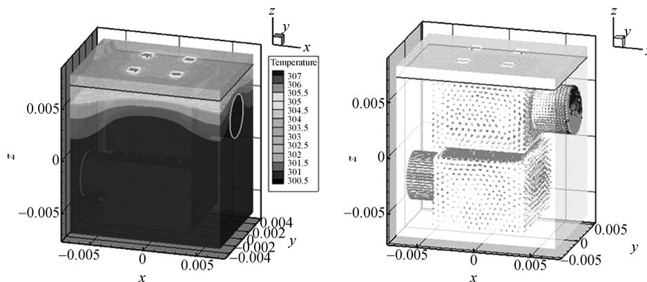
**Figure 12** (a) Temperature distribution in micro jet device; (b) velocity distribution in micro jet device.
