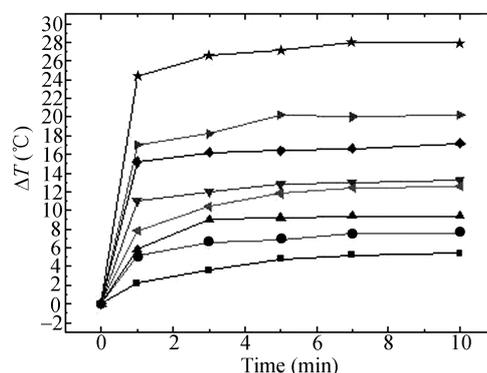
**Figure 8** LED surface temperature with time at different input power and micro pump flow rate. ■, 0.6 A, 7.1 V, 10 mL/S; ●, 0.6 A, 7.1 V, 2.5 mL/S; ▲, 1 A, 7.4 V, 10 mL/S; ▼, 1 A, 7.4 V, 2.5 mL/S; ◄, 1.5 A, 7.9 V, 10 mL/S; ►, 1.5 A, 7.9 V, 2.5 mL/S; ◆, 2 A, 8.2 V, 10 mL/S; ★, 2 A, 8.2 V, 2.5 mL/S.
