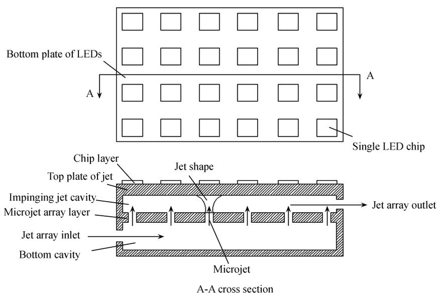
**Figure 2** Microjet array cooling device.
