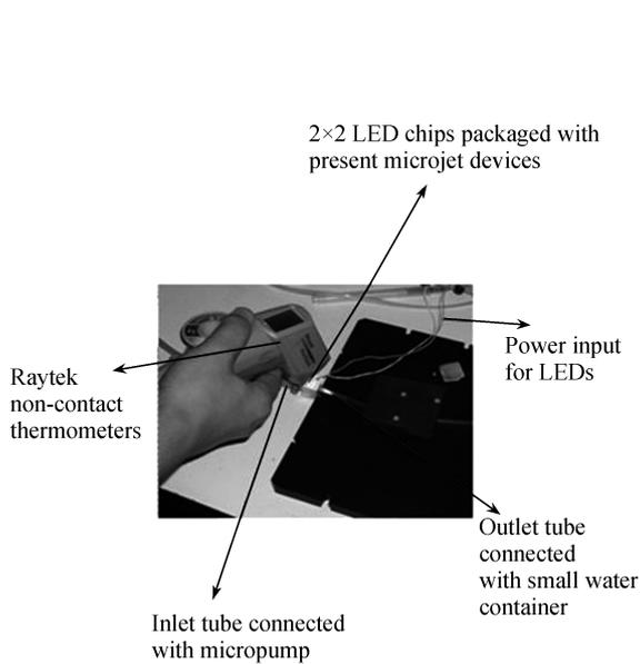
**Figure 4** Surface temperature measurement of LED chips.
