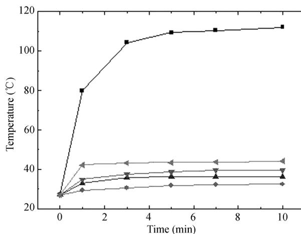
**Figure 7** LED surface temperature with time at different input power and cooling conditions. ■, 0.3 A, 6.3 V, no cooling; ♦, 0.6 A, 7.1 V, with cooling; ▲, 1 A, 7.4 V, with cooling; ▼, 1.5 A, 7.9 V, with cooling; ◀, 2.0 A, 8.2 V, with cooling.
