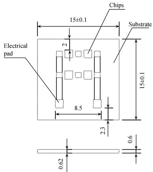
**Figure 5** Detailed size of LED chip layout on substrate.
