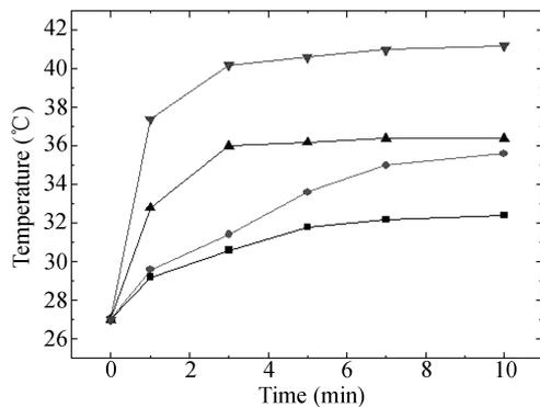
**Figure 9** LED surface temperature variation with time at different fan operation conditions. ■, 0.6 A, 7.1 V, fan operation; ●, 0.6 A, 7.1 V, no fan operation; ▲, 1 A, 7.4 V, fan operation; ▼, 1 A, 7.4 V, no fan operation.
