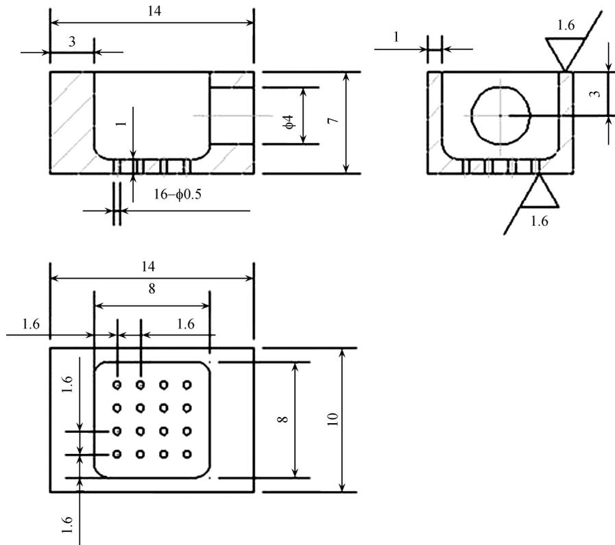
**Figure 6** Detailed size of top cavity of micro jet device used in present experiments.
