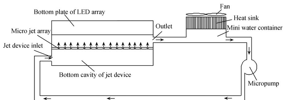
**Figure 1** Present closed microjet array cooling system.
