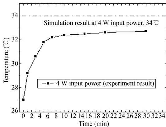
**Figure 11** Temperature comparison between simulation result and experimental result.
