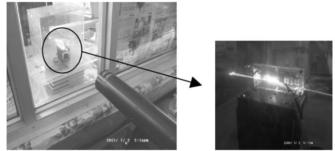
Fig. 9. Photo of measuring mean air velocity in vent by laser Doppler velocimeter.
