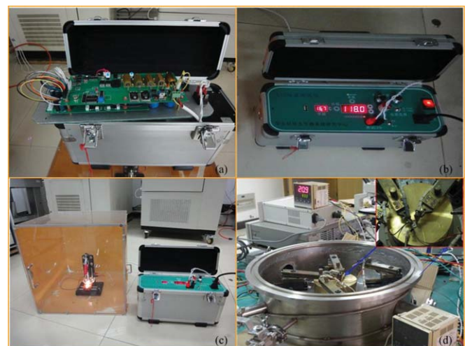
FIG. 2. (Color online) Junction temperature measurement system.
