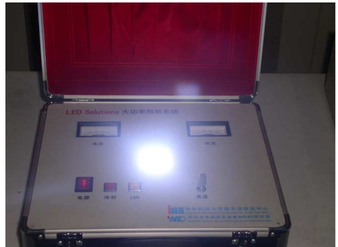
Fig. 15. Demonstration system of 220-W LED lamp cooled by present system.
