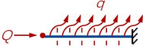
Fig. 2. The 1D heat transfer model of the vacuum flask containing the internal heat source after simplification.
