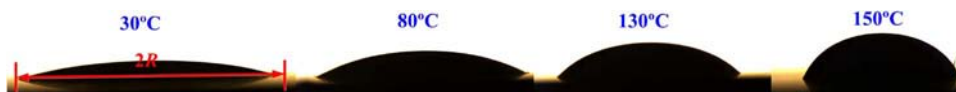
Fig. 4. Side view of the final geometries at 30 °C, 80 °C, 130 °C, and 150 °C, respectively.
