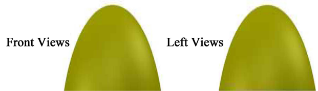
Fig. 6. Front view and left view of phosphor layers in LED module without gold wires.
